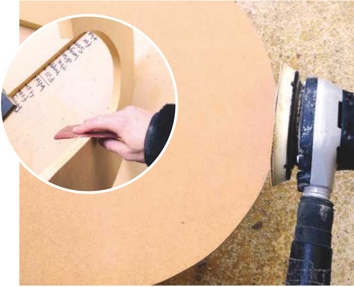
▲ Pic.4 The next step was to sand off the saw marks. I wanted my light to have an antique looking effect, but I didn't want any saw marks showing. First off, I ran round the shape with my orbital sander, moving onto hand sanding for the tighter curves. I also made sure to round over the edges a little, just to soften it up slightly
